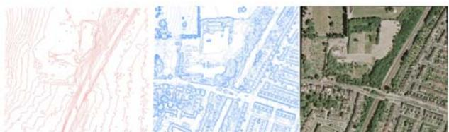
The data has been provided by InfoTerra and BlueSky, revealing their capability to build complex terrain and contour maps using LiDAR imagery plotting both the underlying ground contour (with buildings and vegetation removed) and a more complex image showing the contours with them in place (blue outlines).
